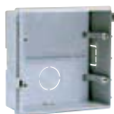
Type: 6149 Description: flush-mounted back box for 6600 series interphones and monitors Material: copolymer Dimensions (WxHxD): 136x136x59 mm
